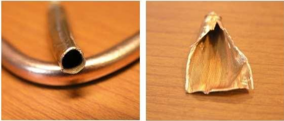
Figure 11. Grooved Wick Type Heat Pipe [10]
