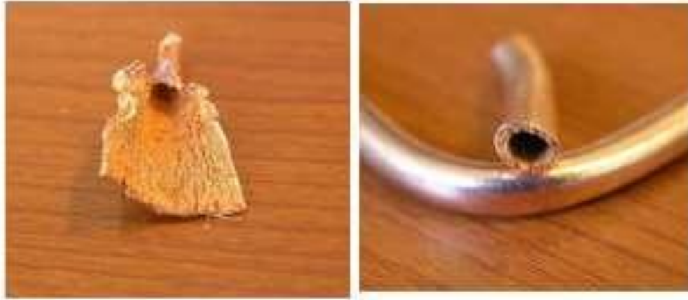
Figure 13. Metal Sintered Powder Wick.
