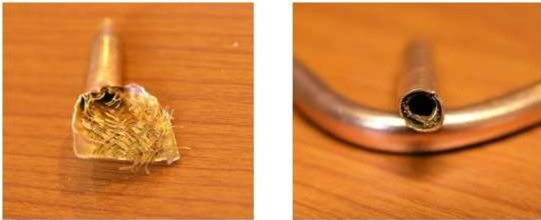
Figure 12. Metal Mesh (felt) Wick Type.
